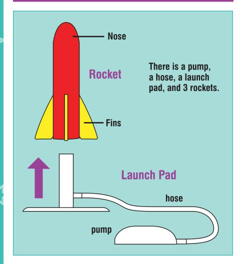
You have an air powered rocket which is subjected to the same forces in flight as a plane; gravity (or weight), thrust, lift and drag.
